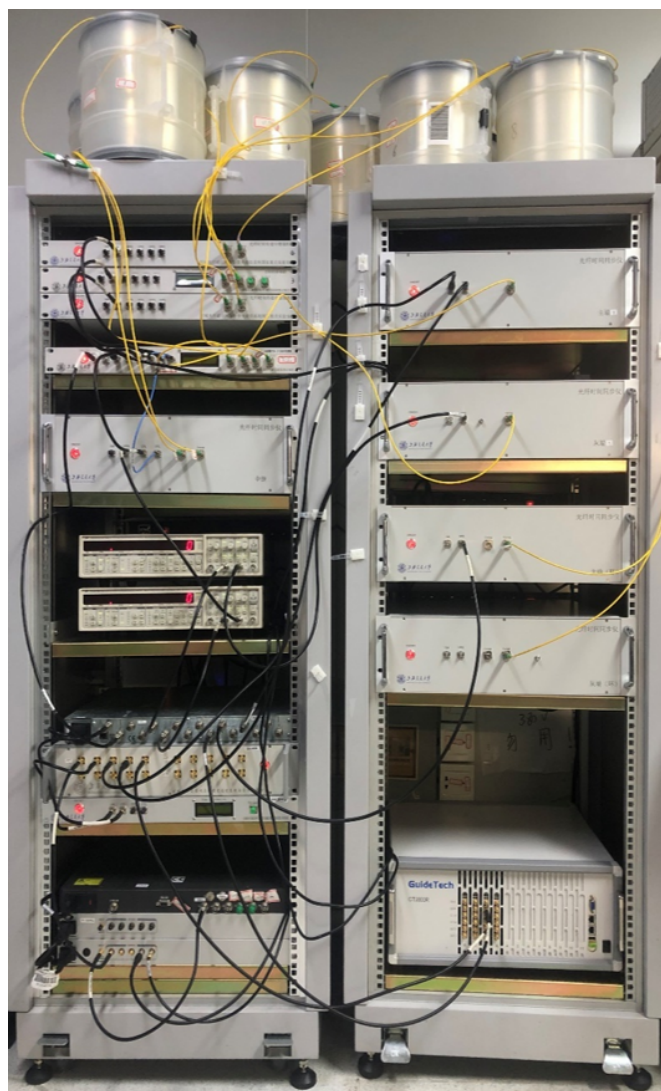
Fig. 2. The photo of the fiber-optic time synchronization system.
